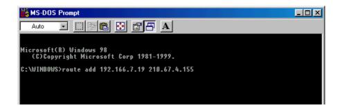
7. At the MS-DOS prompt type: route add 192.166.7.19 210.67.4.155. Then hit enter. The first string is the IP Address and the second string is the Gateway Address.
